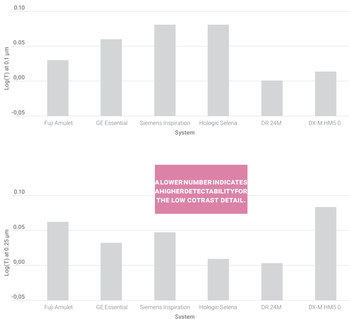
FIGURE 3 CDMAM threshold gold thickness for 0.1 (top) and 0.25 mm (bottom) disks in CDMAM 3.4
